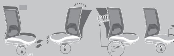
Sincro autorregulable / Self-adjustment synchro / Synchro automatique
